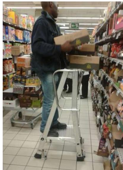
A useful technical support: the tool combines a platform for goods and a table support for parcels, both of which are variable in height. This facilitates the placing of products on shelves by reducing the effort required by employees. It is especially useful for goods placed on higher shelves. The tool also allows employees to sit down whilst placing products on the lower shelves. Overall, this reduces the risk of MSDs.
